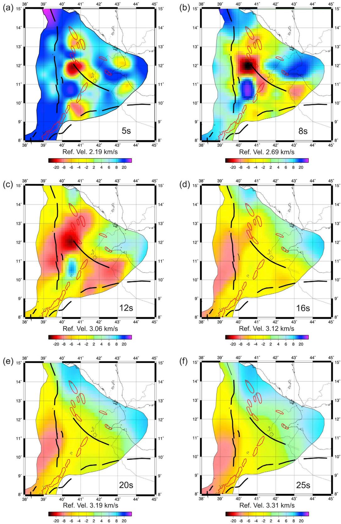
**Figure 2.** (a–f) Group velocity maps at the indicated periods in percentile deviation from the average velocity; areas for which the resolution length is larger than 100 km are in white. Major faults are marked as black lines.
